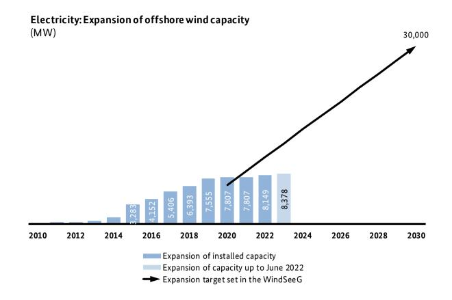
Figure 15: Expansion of offshore wind capacity
