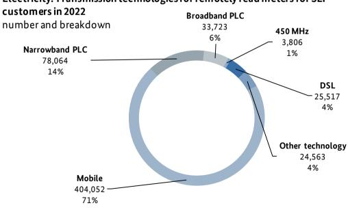
Electricity: Transmission technologies for remotely read meters for SLP
